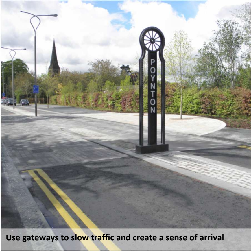
Removal of centre line markings and traditional traffic management measures such as signs and painted marks to reduce vehicle speeds
